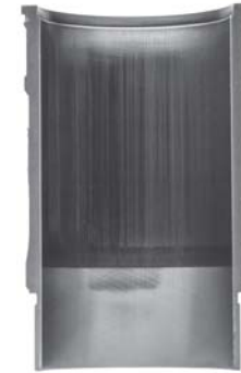
Severely Scuffed Liner
