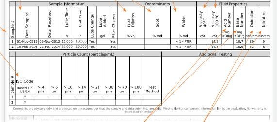
The **ISO Code** is an index number that represents a range of particles within a specific micron range, (e.g. 4, 6, 14). Each class designates a range of measured particles per one ml of sample. This test is valuable in determining large particle wear in filtered systems. This section is only used when a particle count is specified.
